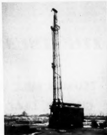
The newest Jet-Piercing machine, the JPM-3, built for the Reserve Mining Company. It will be in operation at Babbitt, Minnesota in the spring of 1952.
